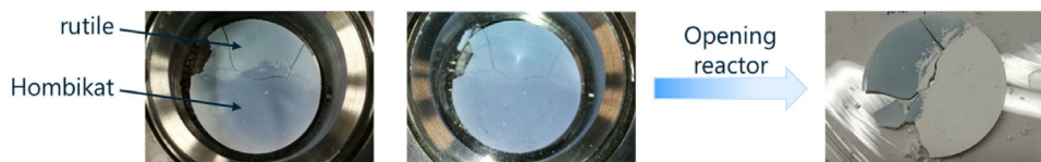
FIGURE 6 | Photodegradation of 2-propanol on a mixed rutile–Hombikat pellet.
