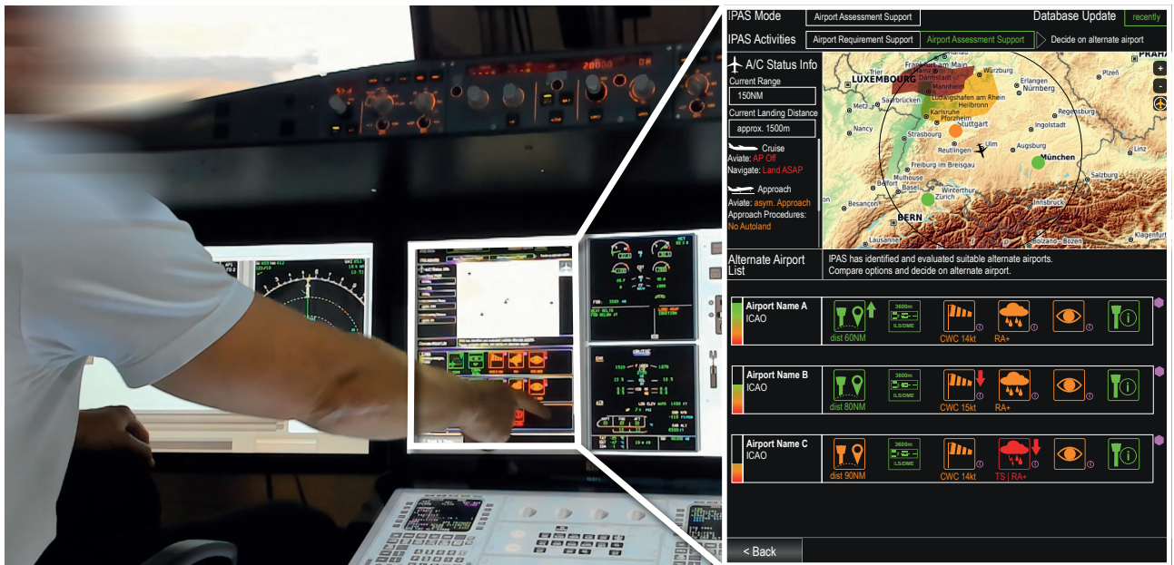
Figure 9.2: AICIS interface integrated into the iSIM showing alternate-airport list, taken from authors publication [81]
