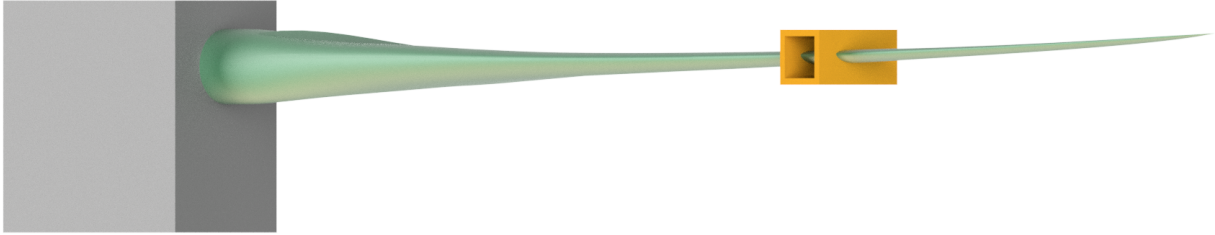
Figure 1. CAD overview of the test setup. The 12.6 m rotor blade is mounted on the test rig with the pressure side facing upwards. The yellow box represents the imbalance fatigue exciter, which is mounted at a radius of R = 7.8 m.
