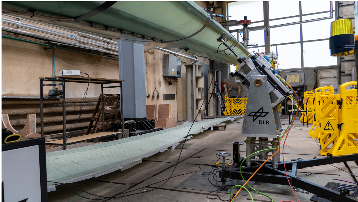
Figure 3. Picture of the APS420 long stroke shaker from SPEKTRA, installed on the rotor blade at R = 3.5 m.
