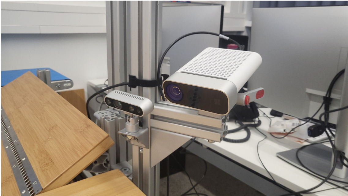
Figure 4.2: The Intel RealSense camera (left) and Microsoft Azure Kinect camera (right), that were used for the pose estimator in this work. They were attached close to the workbench surface, to be able to observe the target object from a close distance.
