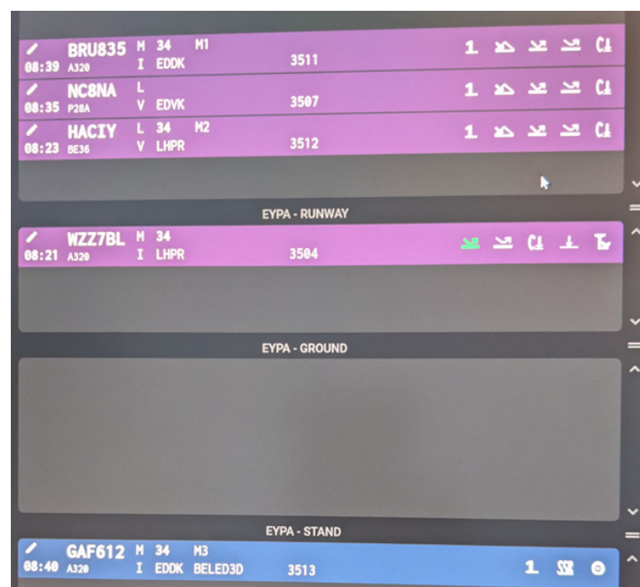
Figure 6. Prototypic electronic flight strips (blue departures; violet arrivals) in different bays (air, runway, ground, stand) with relevant information on the left (estimated time, callsign, aircraft type and weight category, flight rules, runway, destination airport, stand, departure route, squawk) and status icons on the right (e.g., CLEARED TOUCH_GO in green, ENTER_CTR, etc.).
