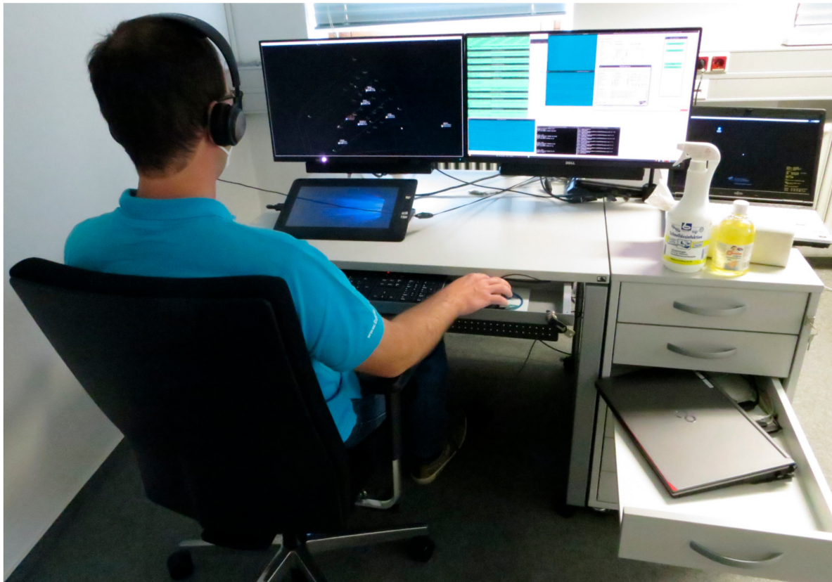
Figure 5. Study participant during simulation trials using an eye-tracking supported attention guidance system for assistant based speech recognition.
