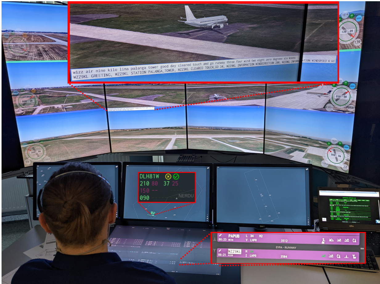
Figure 3.6: ASRU output in (1) an electronic flight strip with colored icons (lower right red box), (2) an aircraft radar label with colored values (center red box), and (3) in an outside view of a multiple remote tower setup with transcribed utterance text and annotated ATC concepts (top red box).
