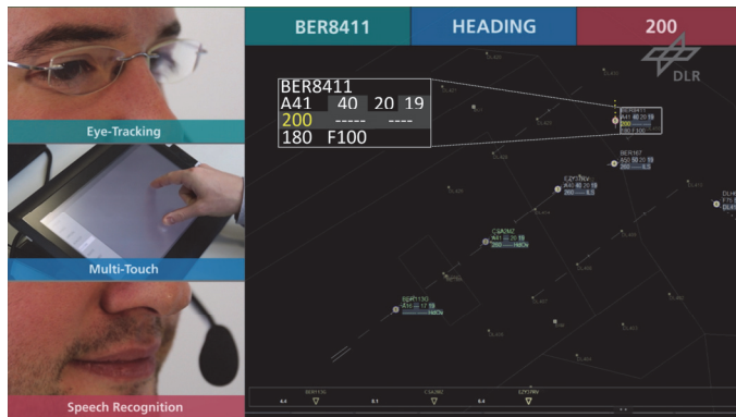
Figure 6. Multimodal prototypic CWP exhibit TriControl
