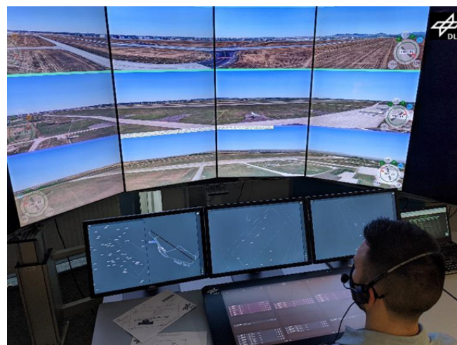
Figure 1. Multiple remote tower environments with a row of monitors per each of the three airports under ATCo control, three radar screens, and the electronic flight strip system that is supported by the output of an assistant-based speech recognition system. The position for Vilnius is always top/left, Kaunas is middle, and Palanga is bottom/right.
