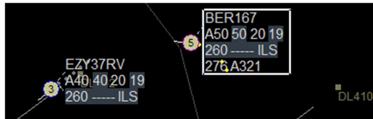
Figure 2. White box around the currently selected aircraft as shown in the radar display.
