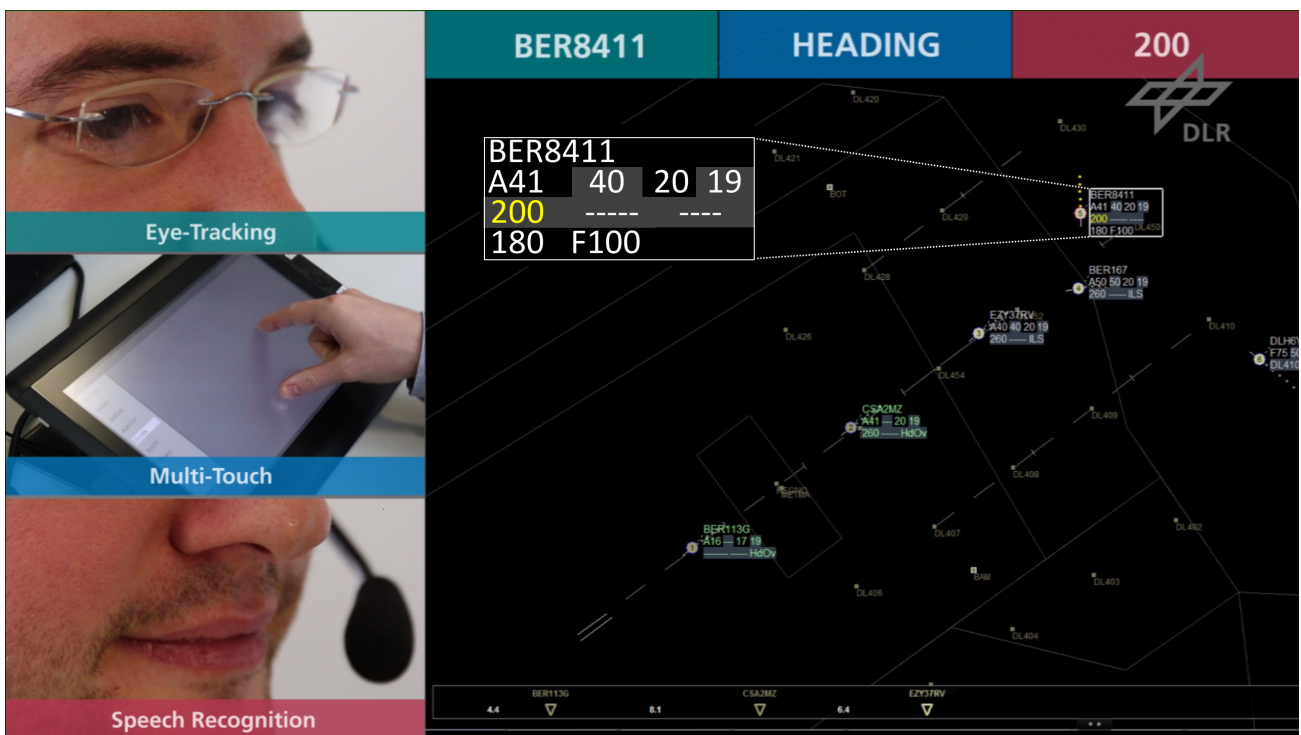
Figure 3.13: Validation setup of the multimodal controller working position prototype TriControl integrating eye tracking, gesture recognition, as well as speech recognition and understanding.
