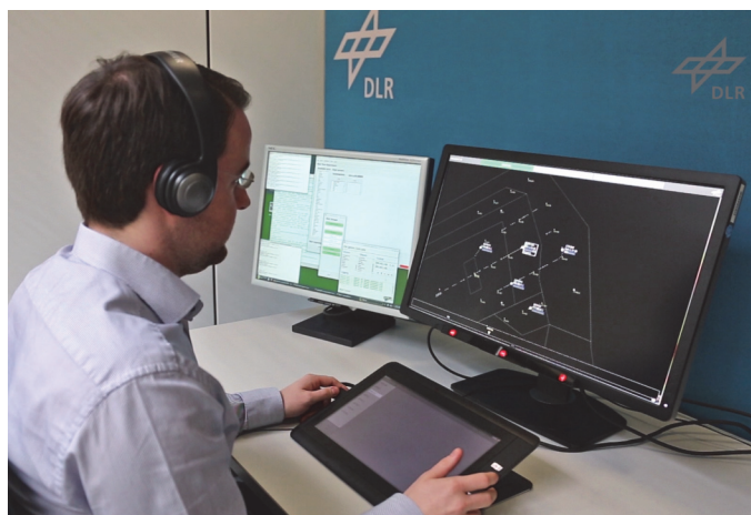
Figure 7. TriControl setup with radar display attached eye tracker, headset, and multi-touch device
