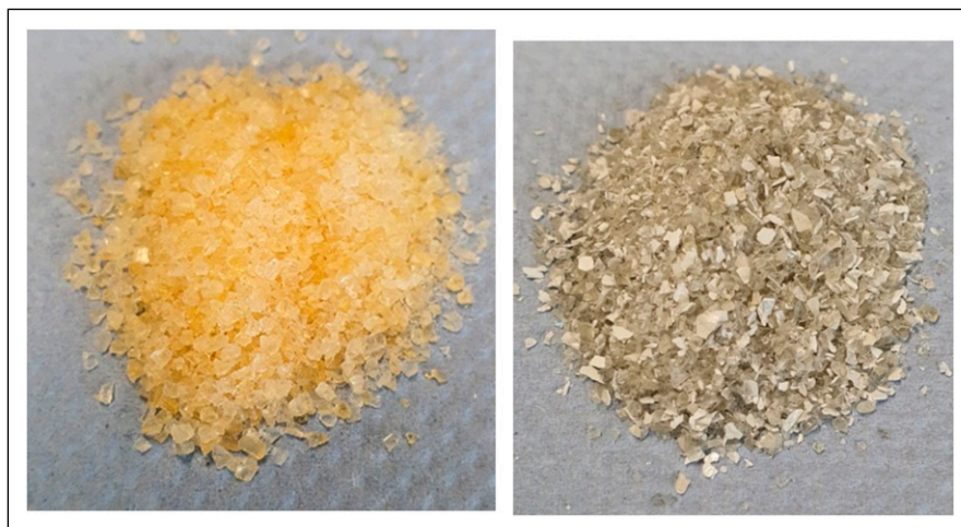
Figure 2. Pre-polymerised recyclate granulates (left) and recovered recyclate granulates (right).
