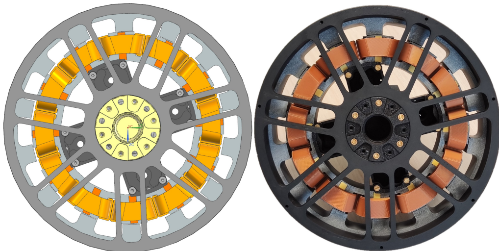
Figure 54: CAD rendering (left) and 3D printed mock-up (right) of prototype FSM machine developed in this study
