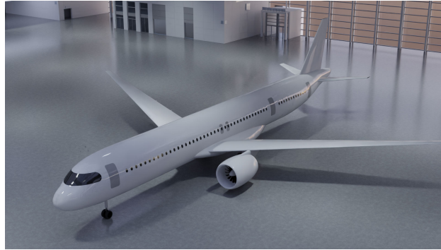
Fig. 10 Three-dimensional view of the DLR-F25 concept ¶ – Credit: DLR (CC BY-NC-ND 3.0).
