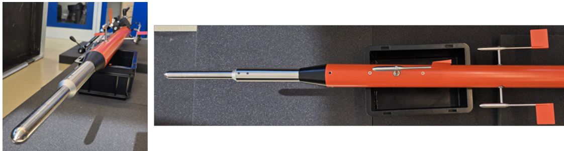
(b) Close up pictures of the air data boom.
