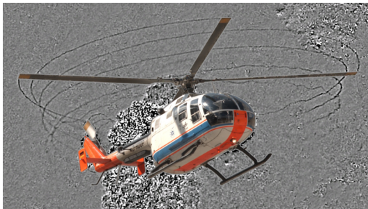
Figure 1.1.: Vortex system of a BO105, visualized with BOS, from Bauknecht et al. (2014)
