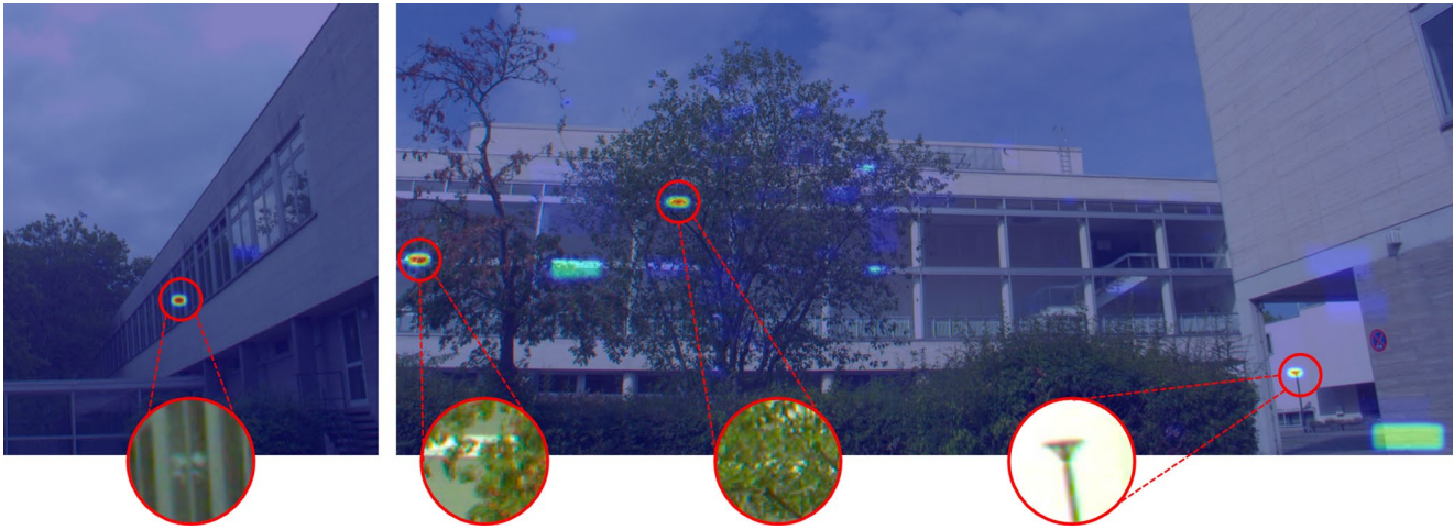
Fig. 4 Spatial distribution of false positives generated by YOLO-FEDER FusionNet (YOLOv8m backbone + DWD-based FEDER features). The distribution is visualized across both camera FOVs of Dataset R1, using cropped regions of the full scenes. Zoomed-in regions
