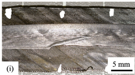
Figure 2.17: Thermoplastic AFP steering-induced out-of-plane wrinkle defect, reprinted from [219] with permission from Elsevier
