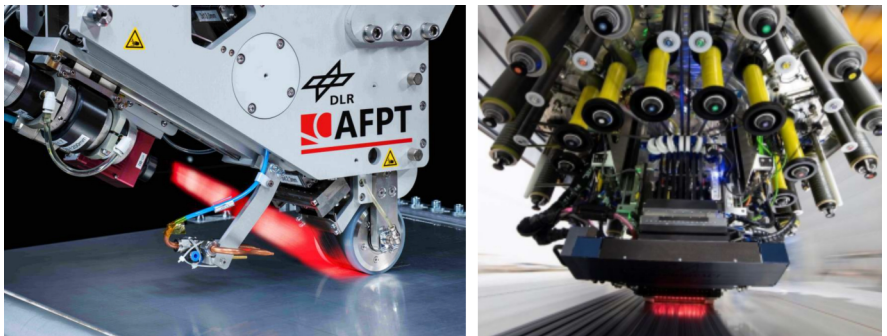
Figure 2.7: Diode laser heating systems: (left) AFP end-effector at DLR Stuttgart with laser optics and animated laser beam, (right) Electroimpact end-effector with variable spot size laser system, reprinted from [77] with permission from SAMPE
