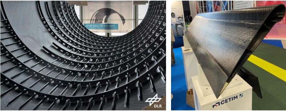
Figure 2.25: Clean Sky 2 in-situ AFP demonstrator components: (left) Multifunctional Fuselage Demonstrator upper shell [289], (right) Krueger wing flap [290]
