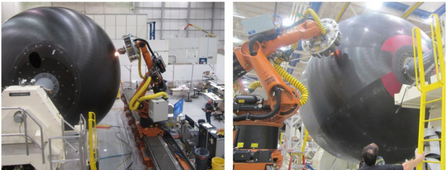
Figure 5.12: NASA and Boeing thermoset AFP composite tank, reprinted from [300] with permission from Elsevier: (left) thermoset AFP process, (right) 0° ply layup
