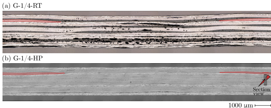
Figure 7.10: Quarter-inch gap defect microsection results
