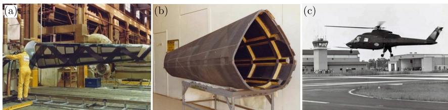
Figure 2.2: Sikorsky ACAP tail cone: (a) Tail cone manufacture using a combination of Filament Winding and Fiber Placement [19, 20], (b) Finished integral tail cone structure [19], (c) Sikorsky S-75 ACAP prototype first flight 1984 [18, 19]
