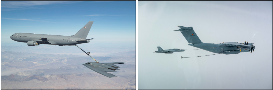
Figure 3.1: Illustration of the air-to-air refueling methods Flying-Boom (left, [149]) and Probe-and-Drogue (right, [1])
