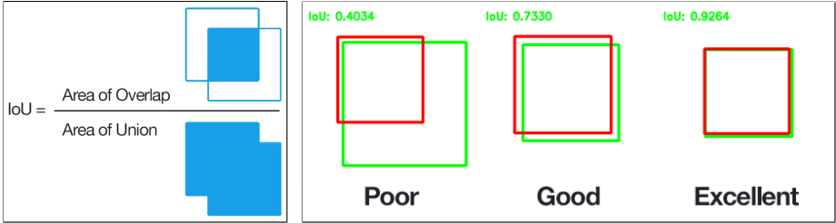
(a) Visualization of IoU calculation. Source: [101] (b) Visualization of different IoU values for two overlapping bounding boxes. Source: [102]
