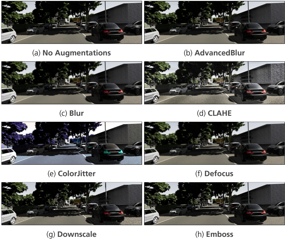
Figure 2.3: Illustration of the effects of the considered image augmentation techniques. Image without augmentations from [146]
