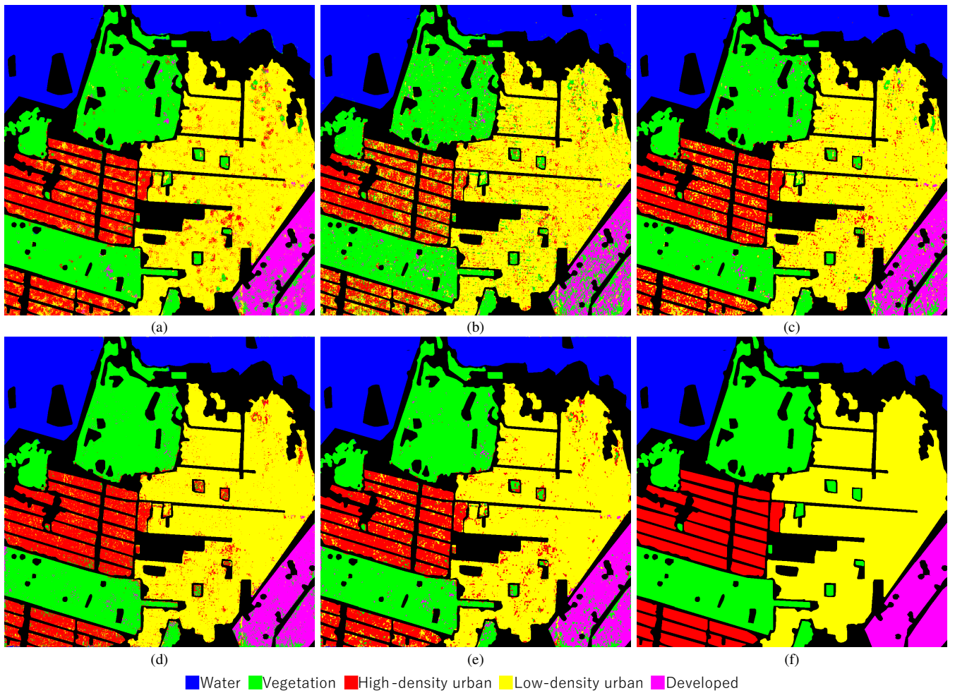
Fig. 5: Classification maps of San Francisco dataset ((a) Refined Lee filter, (b) Extended sigma filter, (c) Pretest filter, (d) 2D QWS, (e) 3D QWS, and (f) Ground truth).
