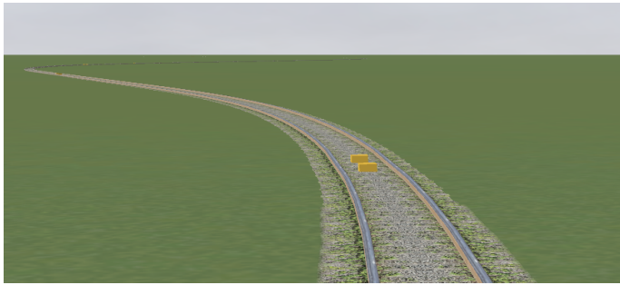
Fig. 4: Output of RGB front-camera sensor from OpenRails. Two balises are shown in yellow on the track.
