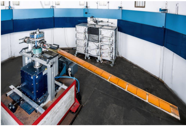
Fig. 22. Investigations of the efficiency of the prototype blade design in centrifugal test rig
