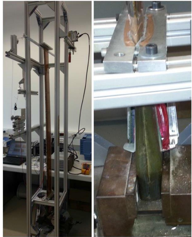
Fig. 14. left: Test rig with rotor blade; right: Rotor blade clamp
