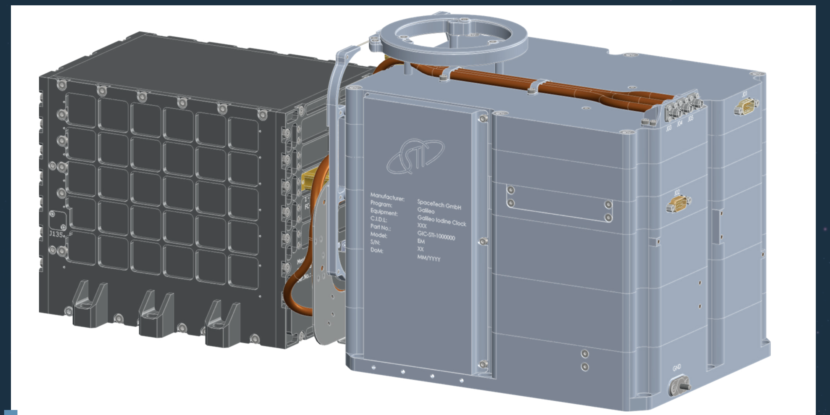
Figure 1: Design of GIC with two independent units, the Iodine Reference Unit (right) and the Frequency Comb (left)
