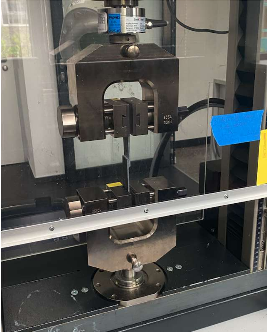
Figure 3.16: Single Lap Shear Test Setup
