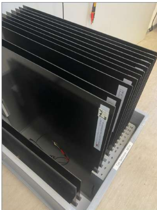
Figure 2.4: set of 10 CFRP plates 66x50 cm, layup [0, \pm 45, 90]_s , thickness of 2.18 mm.
