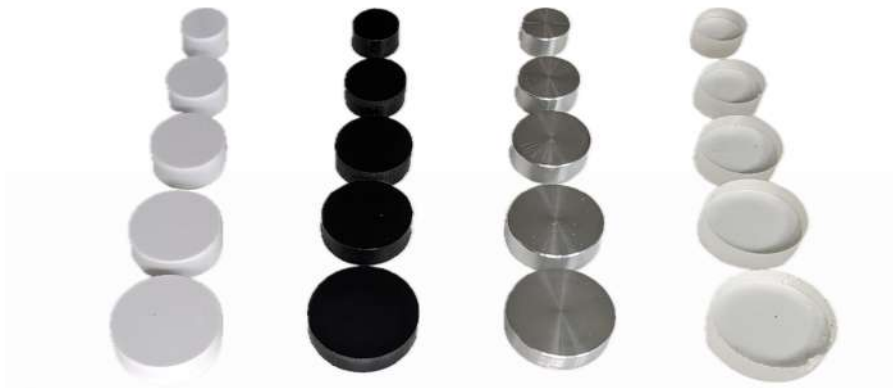
Figure 3.12: different materials and dimensions for the pseudo-damages.
