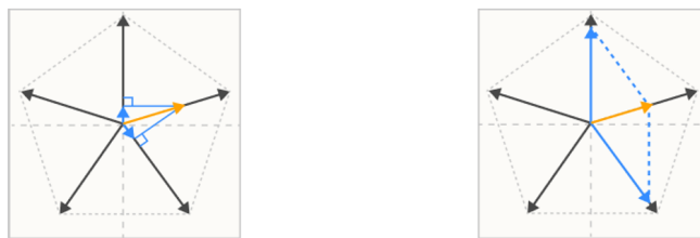
Figure 2.4: Visualization of the superposition hypothesis. An n -dimensional space holding > n features (Elhage et al., 2022)
