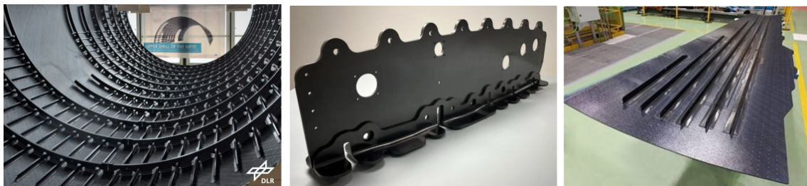
Figure 1: Recent aerospace demonstrators manufactured using CF-LMPAEK: DLR's MFFD (left)[3], Daher's highly-loaded wing rib (centre)[2], and FIDAMC's stiffened morphing wing skin (right)[4]
