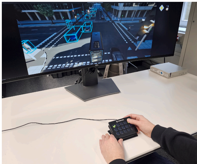
Fig. 2. Participant initiating the left turn at the intersection by pressing one of two available confirmation buttons (green checkmarks on top left and right corner) on the Stream Deck input panel. The top right checkmark is covered by the participant's thumb. (For interpretation of the references to colour in this figure legend, the reader is referred to the web version of this article.)
