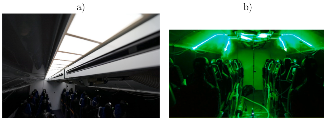
Fig. A.10. (a) Detail image of the vane setting of the slot diffusers. (b) Laser-smoke visualization of the inflow provided by concept Sc1.
