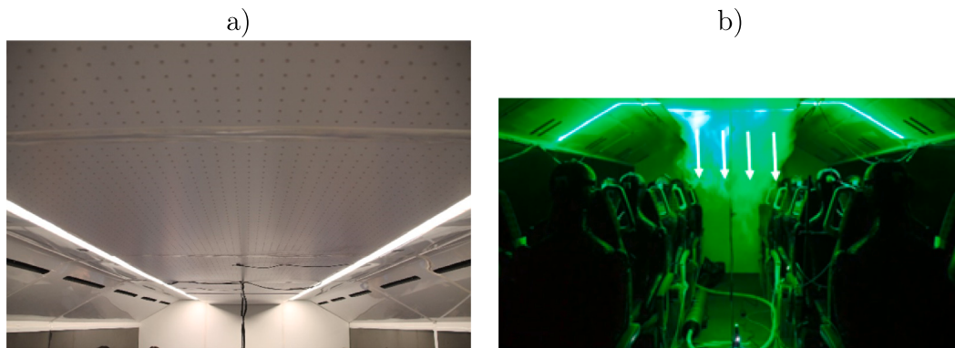
Fig. A.11. (a) Microjet ceiling elements used as supply air inlet in this case. (b) Laser-smoke visualization of the inflow provided by concept Sc2.
