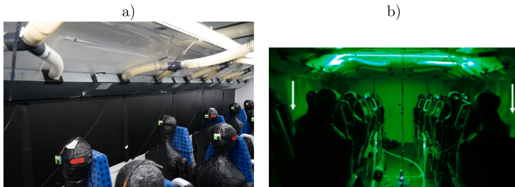
Fig. A.14. (a) Slot diffusers mounted above the window region as inlets for the concept Sc5. (b) Laser-smoke visualization of the inflow provided by concept Sc5.
