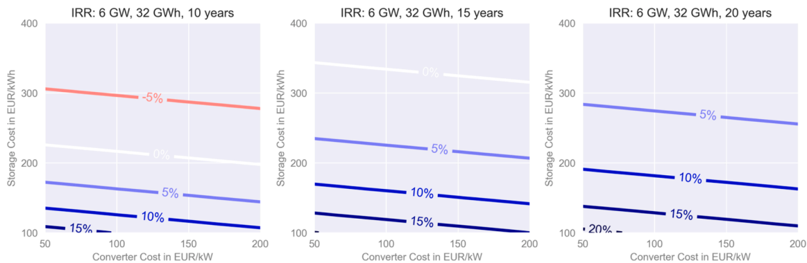
Fig. 10. Internal rate of return (IRR) for the 6 GW and 32 GWh battery storage configuration under operational lifetimes of 10 to 20 years, across the full range of converter costs (50 – 200 EUR/kWh) and storage costs (100 – 400 EUR/kWh). Positive IRR indicates profitable investment assuming constant annual cash flows from day-ahead market arbitrage.
