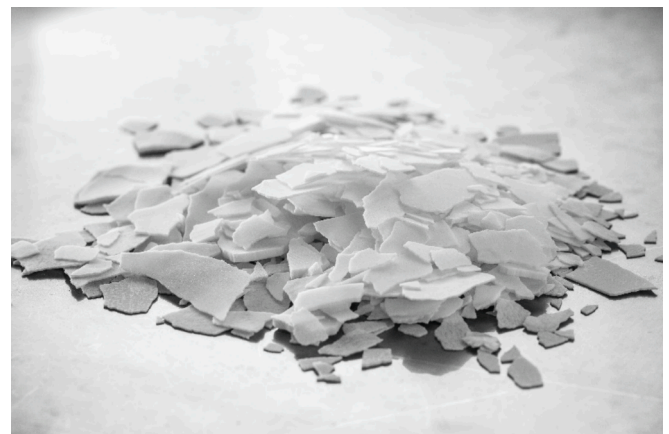
Fig. 11. PCM flakes after being scraped off the rotating drum.
