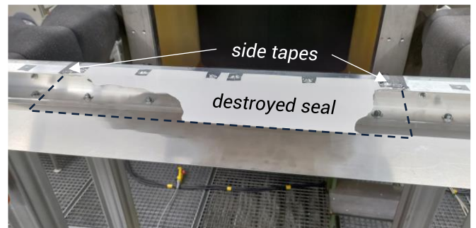
Figure 10: Polystyrene seal after a test run in December 2024.
