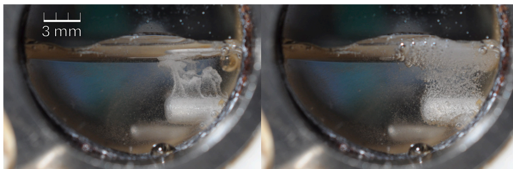
Fig. 5. Images of counter electrode during cyclic voltammetry (FV_Eu_N2) at different moments: cathodic peak C (left) and cathodic limit CL (right).
