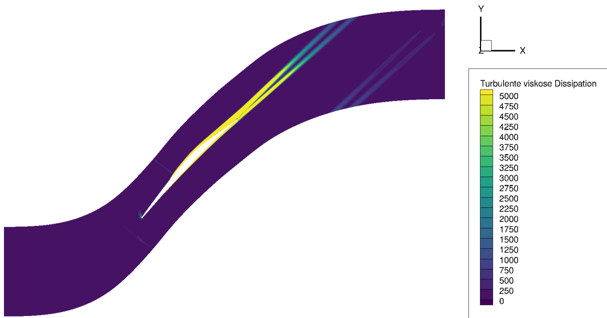
Abbildung 4.3: Lokale turbulente Dissipation D_t in W/(Km^3)
