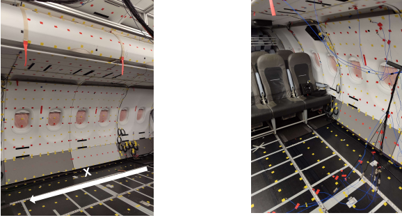
(a) Panel instrumentation. (b) Slice measurement concept.
