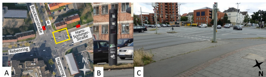
Fig. 2. Application Platform for Intelligent Mobility (AIM) Research Intersection in Braunschweig, Germany. A: Aerial image of AIM Research Intersection (yellow: area of interest for this analysis; red: camera systems used in this analysis, with example in Fig. 2B); B: Stereo camera system; C: Perspective view of the crossing scenario.
