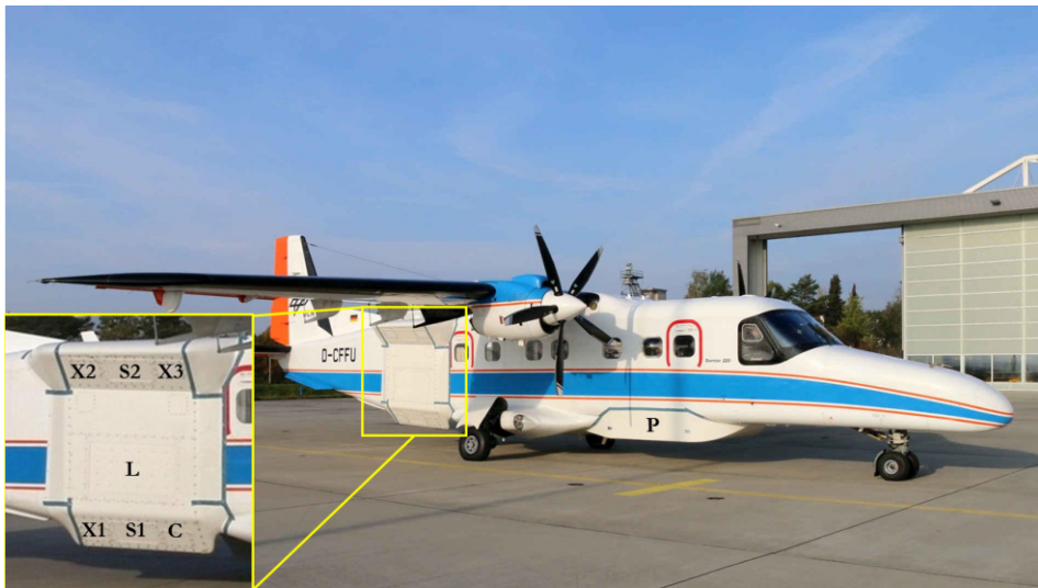
Figure A.4: DLR research aircraft Dornier DO 228-212 equipped with the F-SAR system. The highlighted detail shows the antenna carrier mounted on the fuselage.
