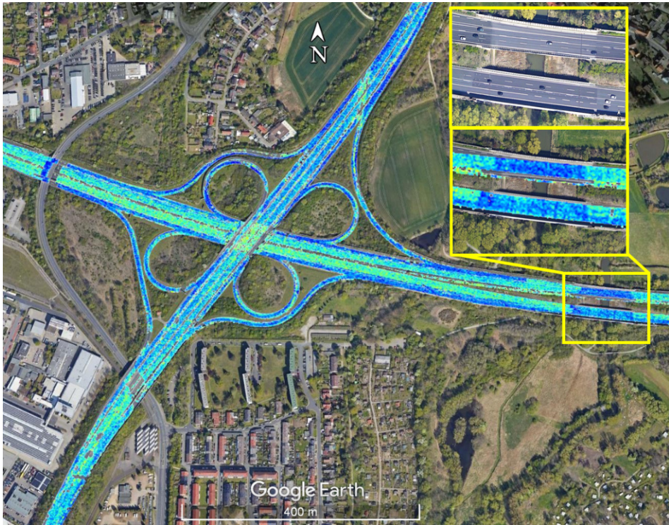
Figure 5.12: h_{\text{rms}} image from a TS-X HH polarised dataset for the A2-A391 motorway crossing in Braunschweig.
