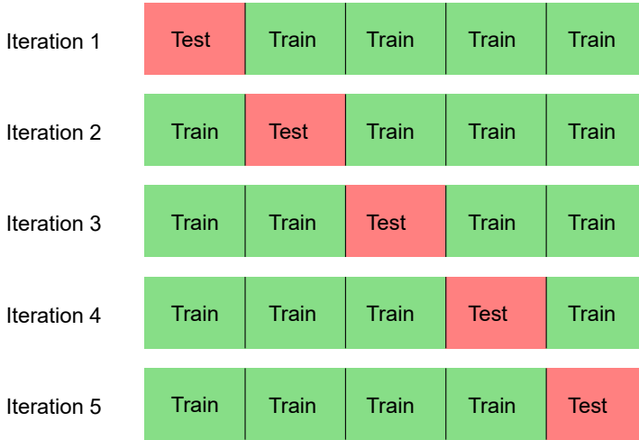
Figure 4.1: Scenario example for K-fold cross-validation in which K = 5 .
