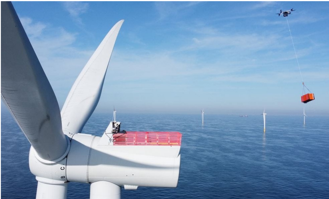
Figure 2.14: FlyingBasket FB3 UAV approaching an Offshore Wind Turbine with Equipment [95]
