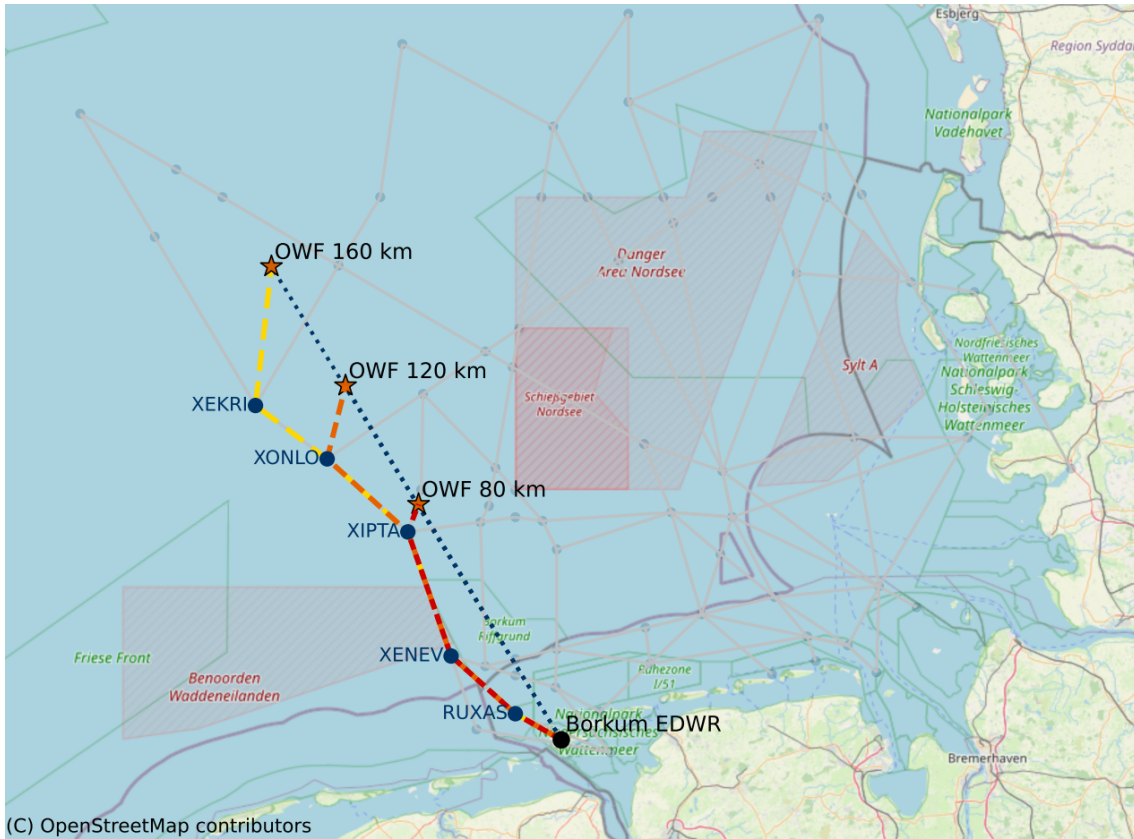
Figure 4.17: Comparison between direct Flight Paths and predefined Waypoint-based Corridors for three Offshore Wind Farms at different Distances from Borkum EDWR
