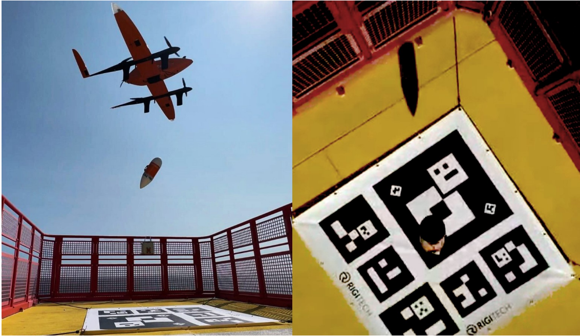
Figure 2.15: UAV dropping a Payload Container on the Winching Area of an Offshore Wind Turbine [100]
