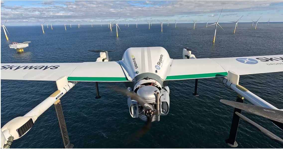
Figure 1.2: VTOL Cargo Drone approaching an Offshore Wind Farm, Source: RWE [20]
