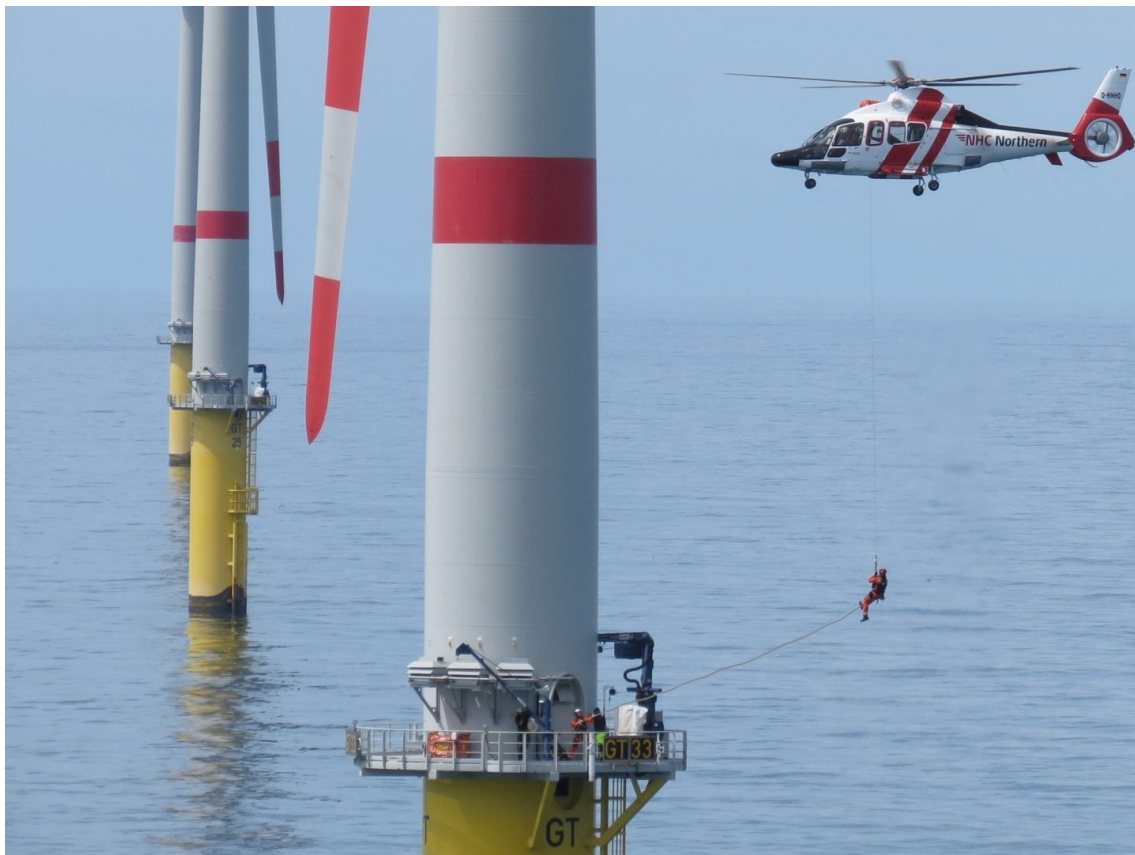
Figure 2.12: HEMS Operation in an Offshore Wind Farm[80]
