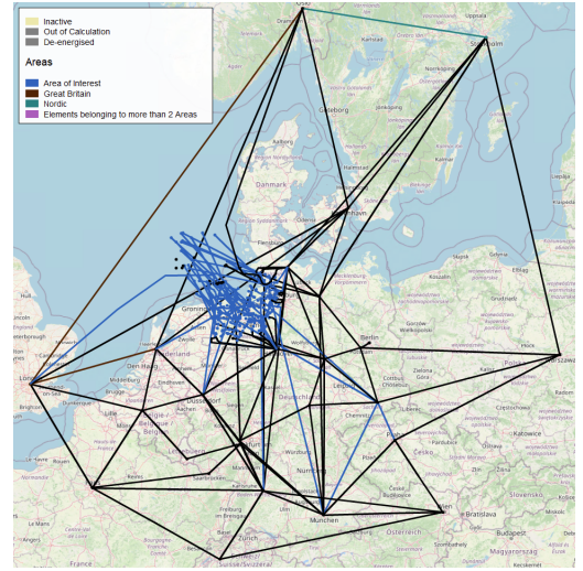
Fig. 5. Resulting PowerFactory grid model, showing region of interest (blue) and simplified (clustered) surroundings (green/black). Background © OpenStreetMap contributors.
