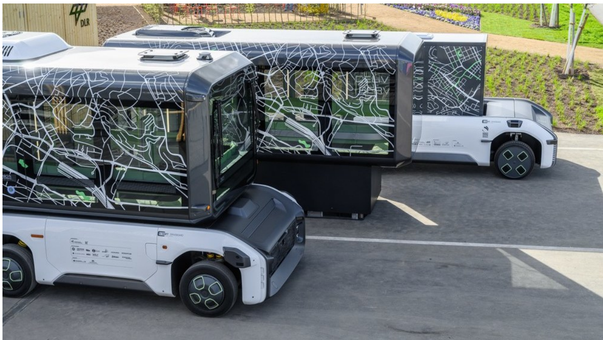
Fig. 2. The U-Shift as a minibus (front), as a goods transporter (rear), together with the single passenger capsule (center). Credit: DLR (CC BY-NC-ND 3.0)
