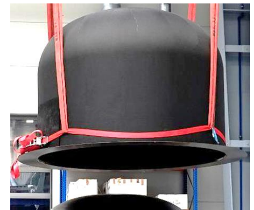
\text{Ø} 1,9 \text{ m} Autoklave Infusion Outer-Tank
