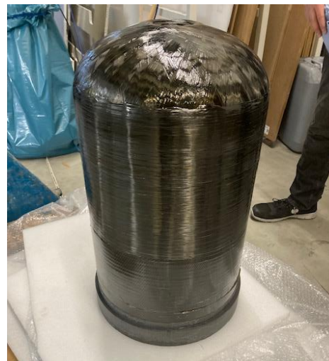
Inner Ø 0,4 m Wet-Filament-Winding (Cryo-) Inner-Tank
