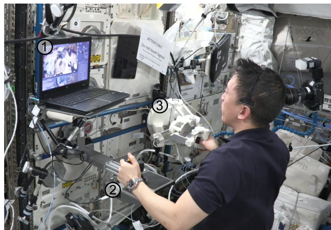
Fig. 1: NASA astronaut Jonny Kim performing a sample collection task, by operating a heterogeneous team of robots from the ISS. He is using a Graphical User Interface (GUI) (1), a joystick (2) and a 7 Degrees-of-Freedom input device with force reflection (3) to command the robots. Image credit: ESA/NASA
