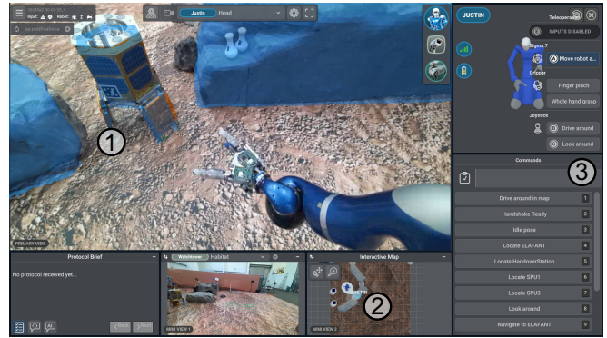
Fig. 3: The GUI displays information about the robots, such as the robots’ known objects and their positions in the form of augmented reality overlays (1) and the robots’ positions in the map (2). It can also be used to give task level commands (3) to the robots.
