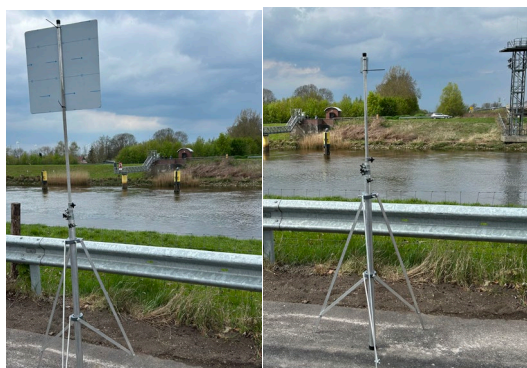
Figure 5. Measurement setup of different plate sizes and corresponding LiDAR recordings
