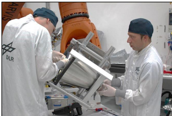
Figure 6: Robot assisted tip integration at the Nose Cone
