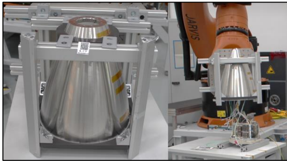
Figure 5: Nose Cone in MGSE cage (left), attached to the robot arm (right)
