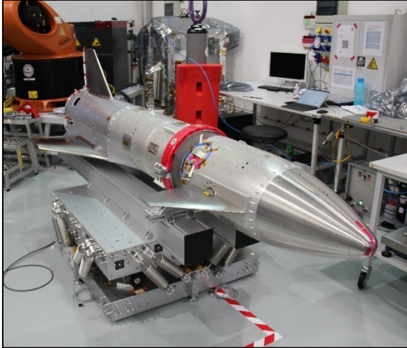
Figure 3: Mass Properties Measurement by Resonic (SM)
