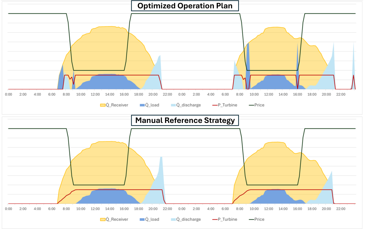
Figure 15: Comparison of optimized operation plan from the operation management agent against manual reference strategy on two subsequent sunny days. \dot{Q}_{\text{Receiver}} : Thermal power absorbed at the receiver based on measured DNI; \dot{Q}_{\text{load}} : Charging power of the thermal storage; \dot{Q}_{\text{discharge}} : Discharging power of the thermal storage; P_{\text{Turbine}} : Electric power output of the turbine; Price: Time-dependent electricity price on the energy market
