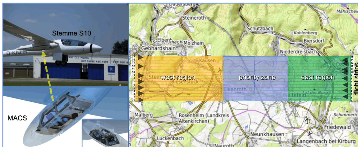
Fig. 3 The research aircraft (a Stemme S10 motor glider, top-left) was equipped with the Modular Aerial Camera System (MACS, bottom-left) mounted in one of its underwing pods. This system was used for data acquisition. The flight plan (right) displays the locations and numbering of the 15 flight strips. GPS coordinates for Weitfeld: 50.72468°N (latitude), 7.92714°E (longitude).
