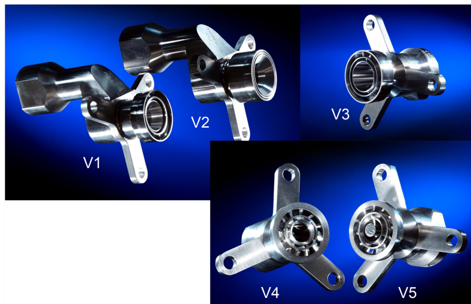
Fig. 2 Tested hydrogen injectors V1–V5 [19]
