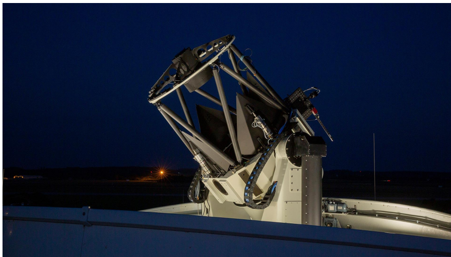
Figure 4.3: OGS-OP Cassegrain telescope with the mirror covers and dome open. This telescope has a pupil diameter of 0.8 m and a central obscuration with 0.3 m.
