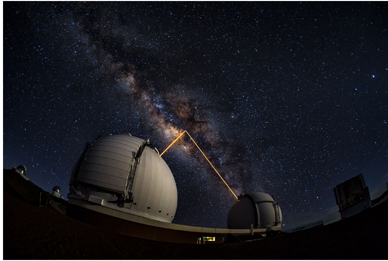
Figure 1.3: Keck Observatory's LGS AO system creating an artificial star to measure for atmospheric distortions. (Credit: Billy Doaner, via Keck Observatory)
