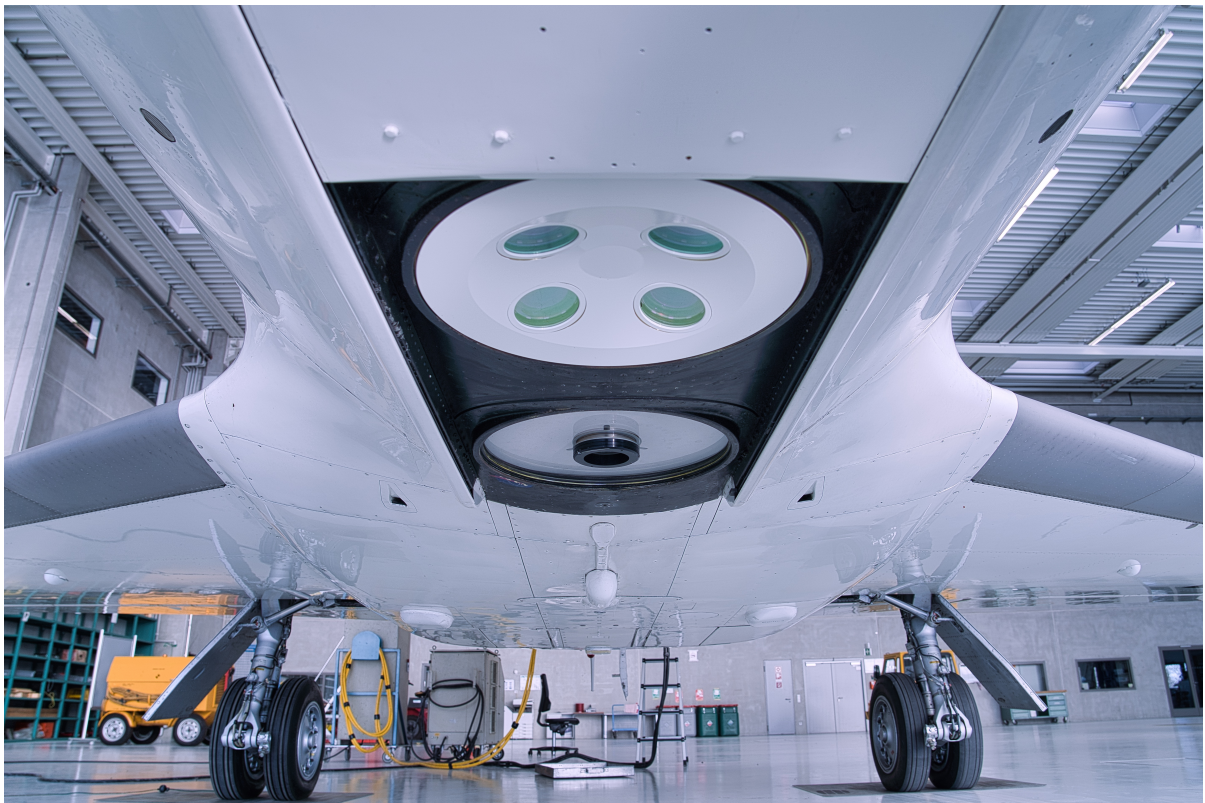
Figure 2.6: LDA Optics installed in the DLR Dassault Falcon 20E research aircraft [37]
