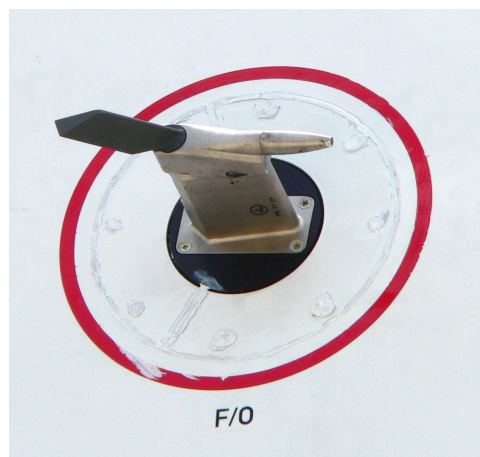
Figure 2.2: Integrated air data transducer on the copilot side of an Airbus A380 [33]
