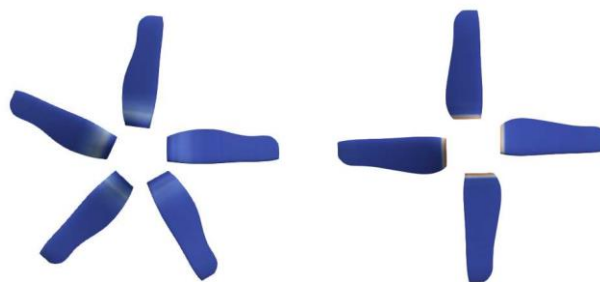
Figure 6: Geometry of the front (left) and aft (right) rotors within Paraview
