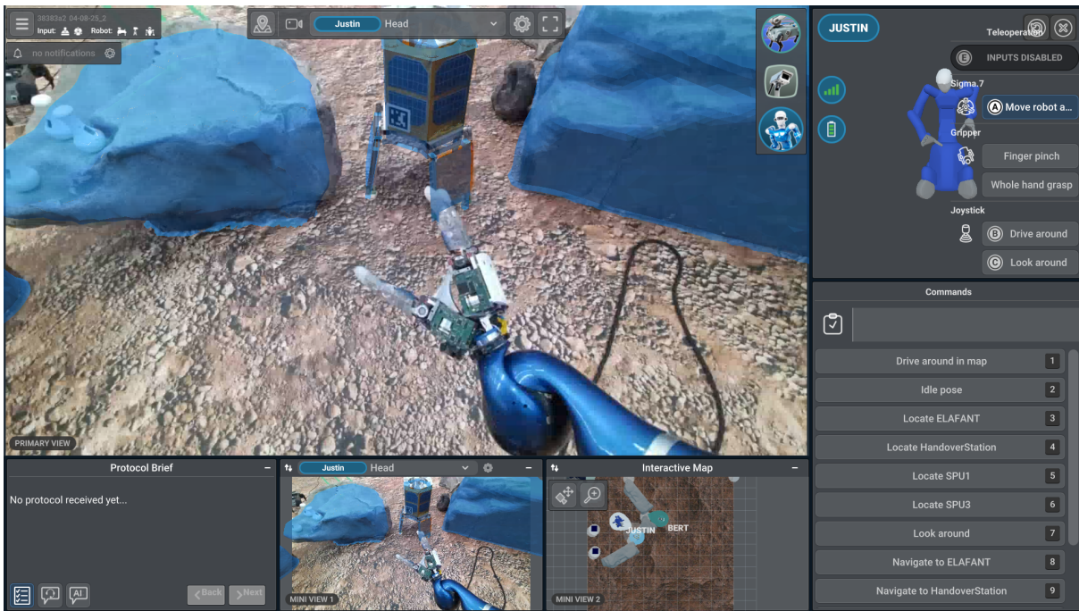
Figure 2.4.: Operator-UI: GUI for task-level commands of the knowledge driven approach from Surface Avatar, picture taken in the user study of [LSL22]
