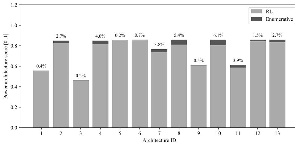
Fig. 11 Comparison of enumerative and RL for optimizing CubeSat's power architecture score
