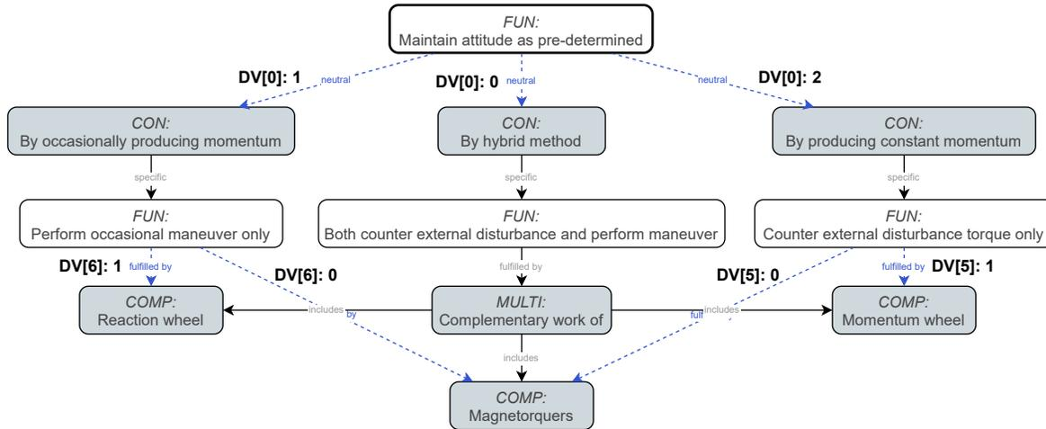
**Fig. 8 Hierarchical architecture decision-making for attitude determination and control subsystem**
