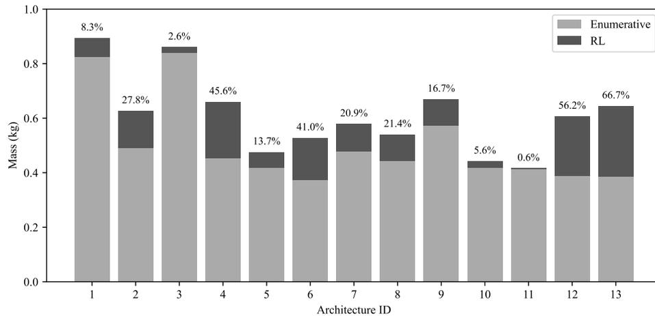
Fig. 10 Comparison of enumerative and RL for optimizing CubeSat's mass
