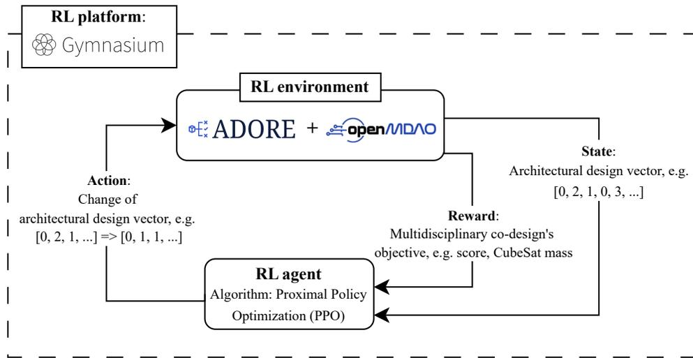
Fig. 5 The workflow of Reinforcement Learning with OpenMDAO and ADORE as environment
