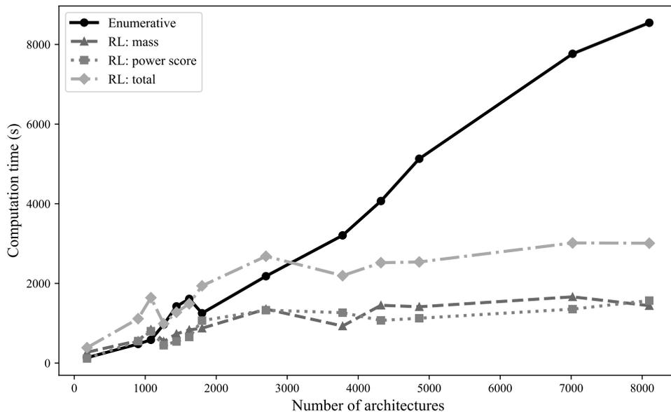
**Fig. 9 Comparison of computation time between enumerative and RL**
