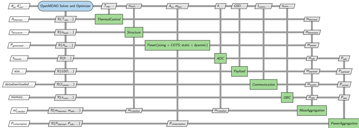
Fig. 12 XDSM of complete CubeSat MDO formulation
