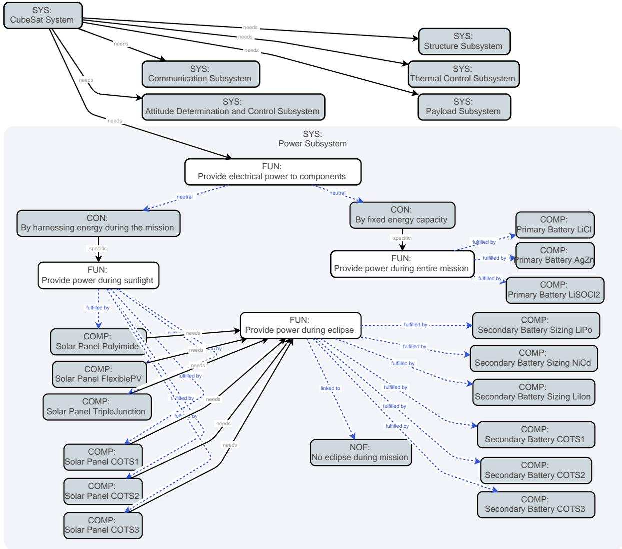
Fig. 2 ADSG of CubeSat and its power subsystem modeling in ADORE
