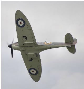
Figure 2.6: Illustration of Spitfire Mk IIa P7350 with near ideal elliptical wing shape. Figure collected from [12]
