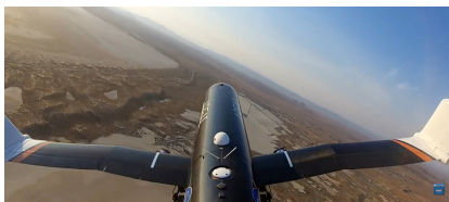
(a) In-flight view of NASA PTERA with flexible wingtips
