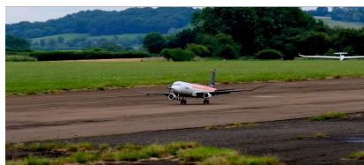
(e) Ground test of Airbus AlbatrossOne
