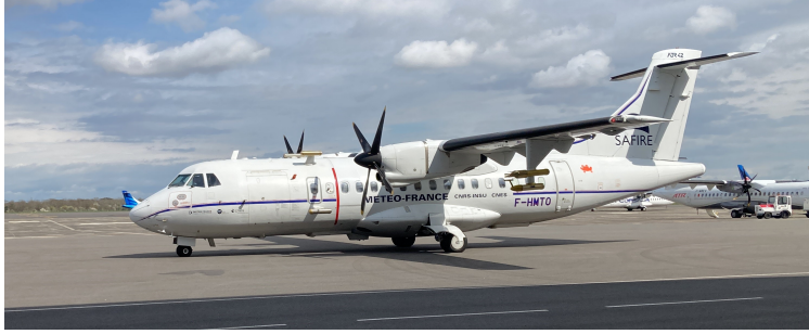
Fig. 1 Safire ATR 42-320 flight test bench (MSN 78): aircraft with all modification for the SENS4ICE European flight test campaign at Toulouse/Franczal airport; credit DLR/Safire.
