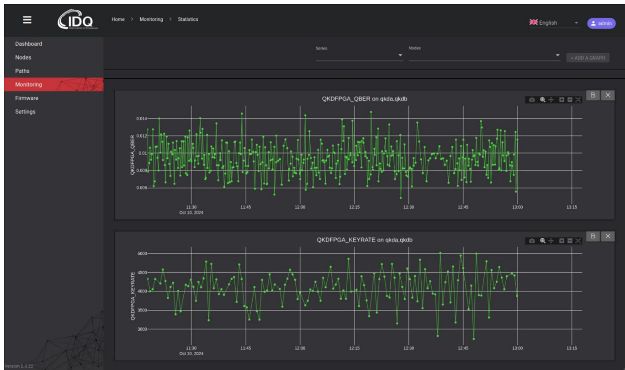
Figure 7 - Example QKD statistics, top: relative error rates [0:1], bottom: key exchange rates in bit/s (avrg. ~4kbit/s)
