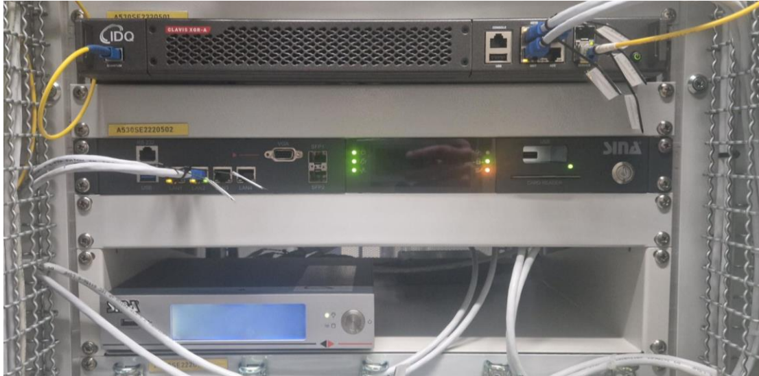
Figure 8 - shows the Clavis XG (QKD device, top) and the modified Sina 30M (grey box, bottom) in the rack
