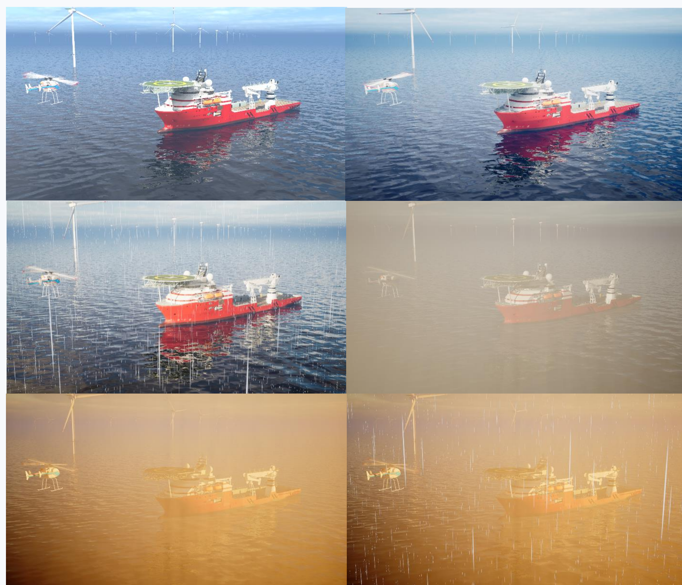
Simulation of different ODD parameters utilizing the SenSim2 framework. Simulation is based on Unreal Engine 5 and can simulate daylight conditions, rain, snow and fog. The simulation framework is also capable of simulating additional sensors, such as Lidar.
