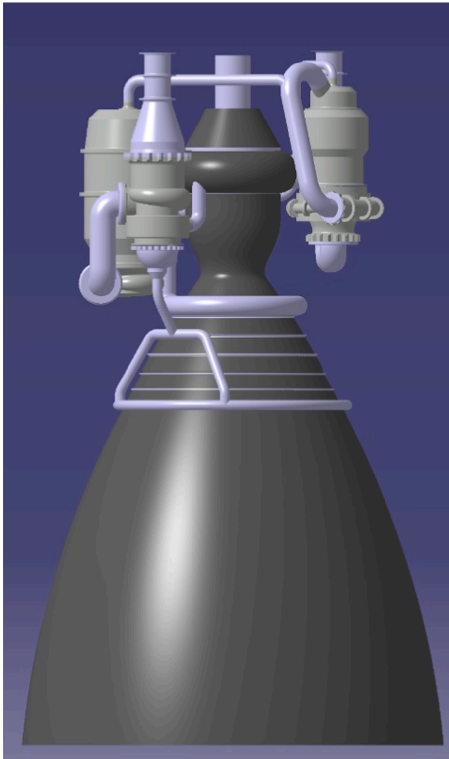
Fig. 2. CAD-drawing of SLME V7 with nozzle expansion ratio 59.
