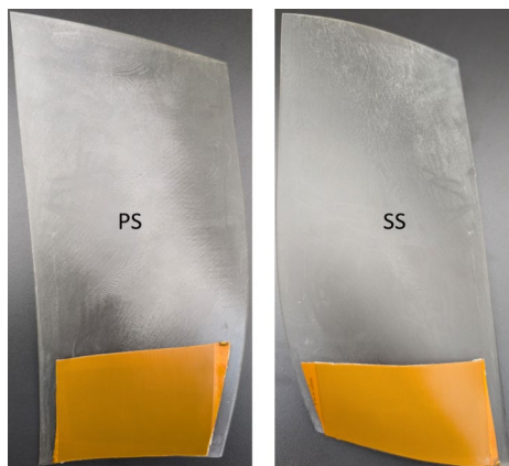
Fig. 12 First actuators of developed array applied onto SE 2 A fan blade
